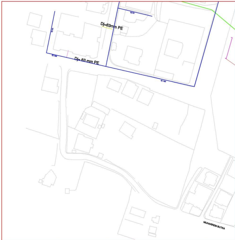
Map 87 –Situation of water supply system in the site
