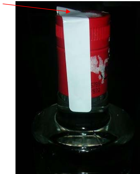
Figure 13 - Not acceptable (Excise Banderol not flat on the top of the cap)
